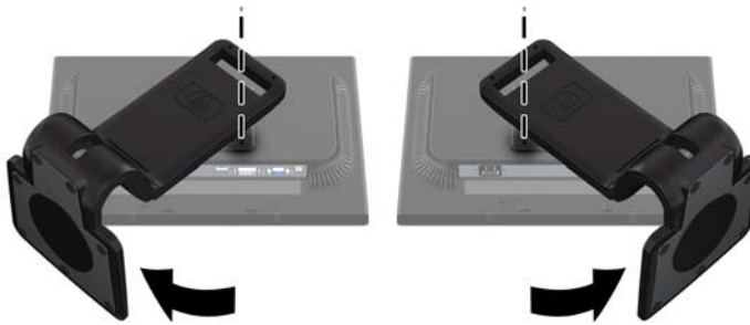
Figure 2-9 Removing the Pedestal Base Screws
